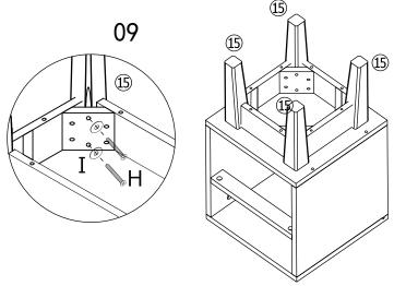
On the basis of "step 08", lock wooden leg (15) on "step 08" with 2 bolt (H) and 2 washer (I), repeat 4 times.
