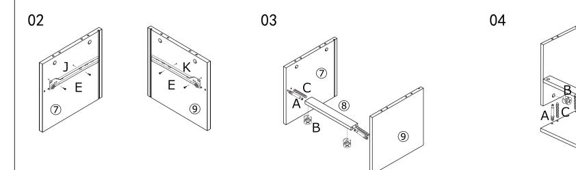
Lock left drawer rail (J) to left side panel (7) with 2 screw (E) and right drawer rail (K) to right side panel (9) with 2 screw (E).
